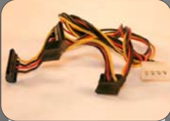
4 pin peripheral power to 4 SAS/SATA device power converter cable
